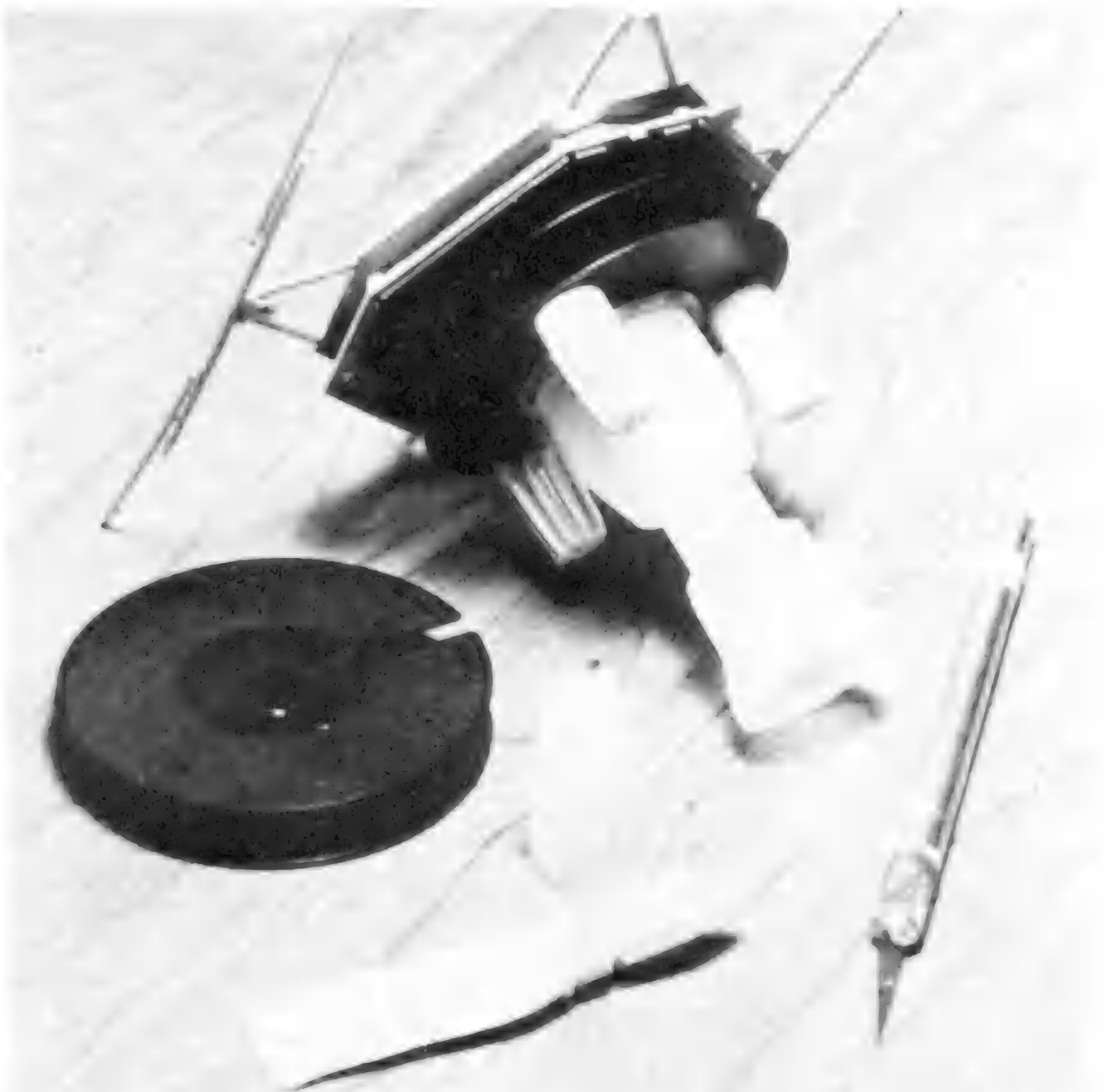
The rocket thruster end of the three-hour-spaceship in early stages of construction. The engine nozzle is the cap of a bottle of Vanish toilet bowl cleaner. Super-8 film reels provide the cylindrical shape.
